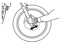
Checking the wheel bearings
