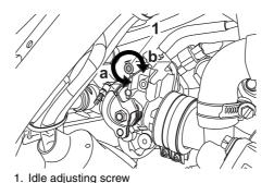
Engine idling speed: 1400–1600 r/min
